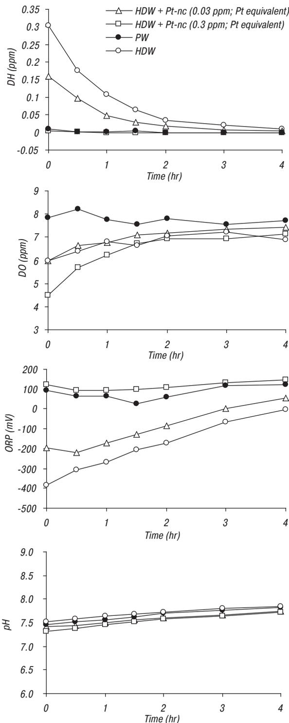
**Fig. 6.** Temporal changes of DH, ORP, DO and pH in cell culture medium prepared with HD-water or purified water and their dependency on the presence or absence of Pt-nc. After preparation of each medium, they were incubated at 37 °C in a humidified atmosphere of 95% air and 5% CO<sub>2</sub>. Then, the parameters were measured at the indicated time points. PW — purified water; HDW — HD-water
