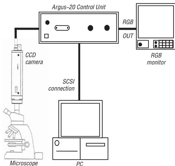
Fig. 2. Block diagram of the image analysis system (Hamamatsu)
