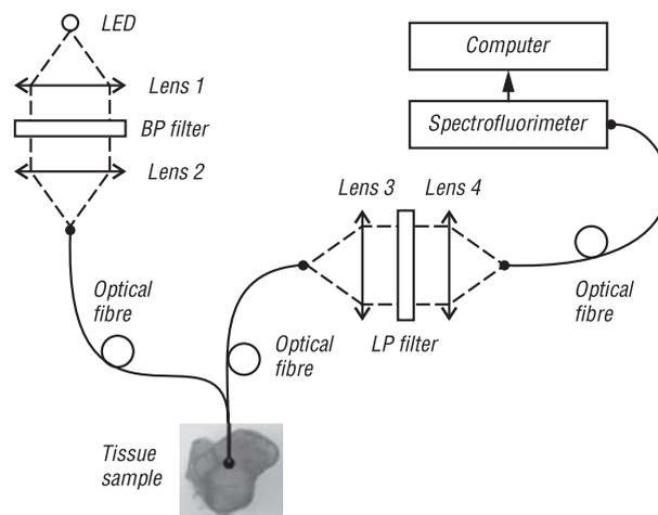
Fig. 1. Schematic diagram of the experimental setup
