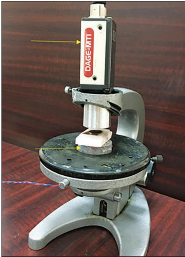
Fig. 1. Schematic of the experimental setup showing a CCD camera over and IR LEDs under the prostate tissue sample
