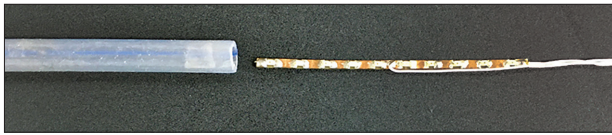
Fig. 1. Prostate illumination tool. Infrared LEDs are mounted on a flexible light guide. The length of the light guide is 50 mm, width 1.8 mm, height 1.68 mm. The light guide is placed into a catheter (shown in the Figure), which is subsequently inserted into the prostatic urethral channel
