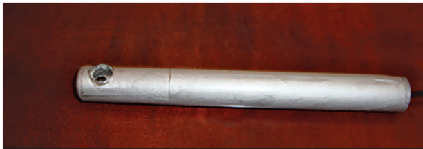
Fig. 2. The device for the visualization of prostate cancer for model experiments. The dimensions of the tool are: the length is 175 mm, and the diameter is 19 mm. The pinhole diameter is 10.8 mm
